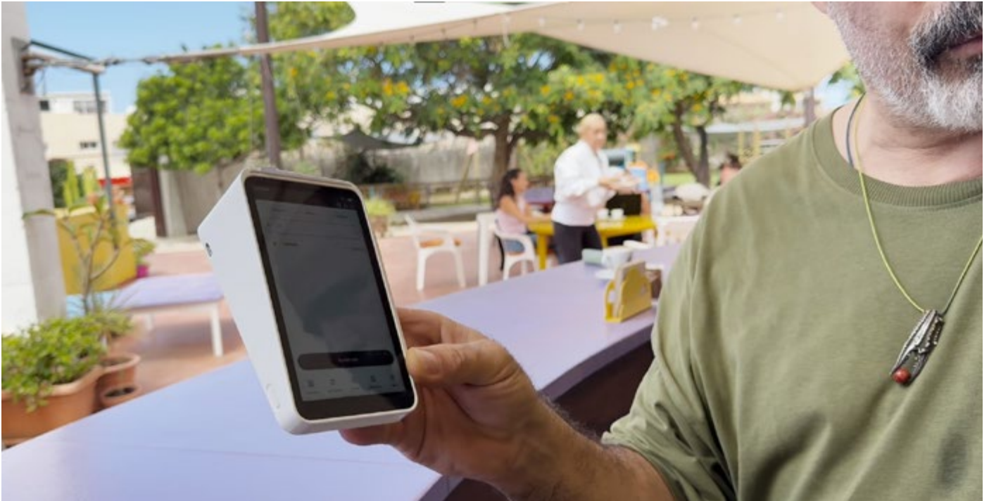
The new mobile terminal in the cafeteria which takes credit card and cash payments, has the menu and also sends orders directly to the terminal in the kitchen.
